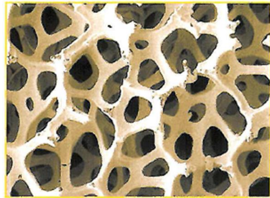
Figure 1: Metallic foam (Magnitude 10^5 )
